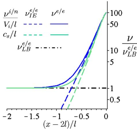
FIG. 1 (color online). Total electron-electron collision frequency normalized to  $\nu_{LB}^{e/e}$  (solid lines) with contributions from Coulomb interactions in a stable plasma (black, dash-dotted line) and from instability-enhanced collective interactions (dashed lines). Two common presheath models are represented:  $\nu^{i/n} = V_i/l$  (blue) and  $\nu^{i/n} = c_s/l$  (aquamarine).
