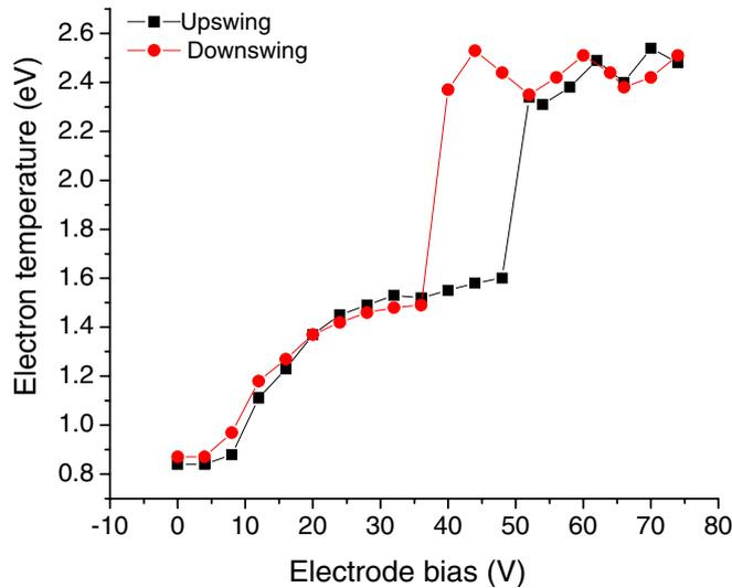
**Figure 8.** Langmuir probes measure a jump in the bulk electron temperature when an anode spot forms, which is indicative of global nonambipolar flow.
