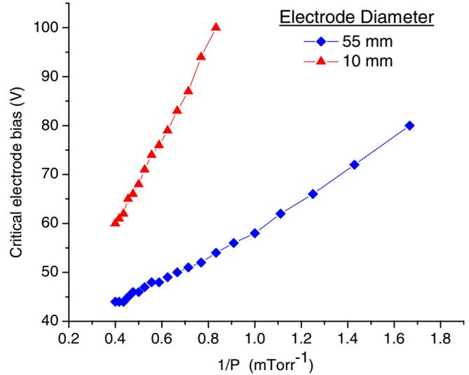
**Figure 5.** The critical electrode bias for onset of an anode spot is shown to be proportional to  $1/P + C$ . Data shown are for electrode diameters of 1 cm (triangles) and 5.5 cm (diamonds).
