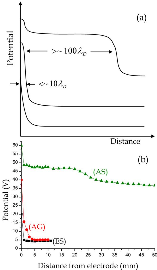
**Figure 4.** (a) Schematic drawing of anode spot (AS), anode glow (AG) and electron sheath (ES) potential profiles. (b) Emissive probe measurements of each solution for an electrode biased at 20V for the electron sheath, 40 V for the anode glow, and 60 V for the anode spot (which in this case was a firerod).
