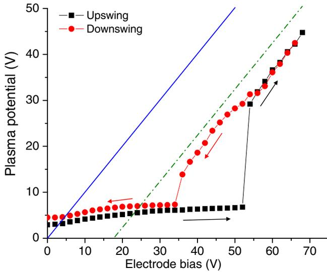
**Figure 7.** Plasma potential versus increasing (squares) and decreasing (circles) electrode bias. The solid line plots plasma potential equal to electrode bias, while the dash-dotted line shows the same less the ionization potential of argon.
