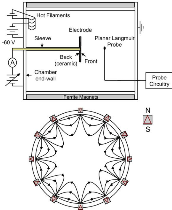
**Figure 3.** Dc anodic double layers and sheaths were generated in front of a one-sided disk electrode submersed in a filament generated argon plasma in a MacKenzie bucket.
