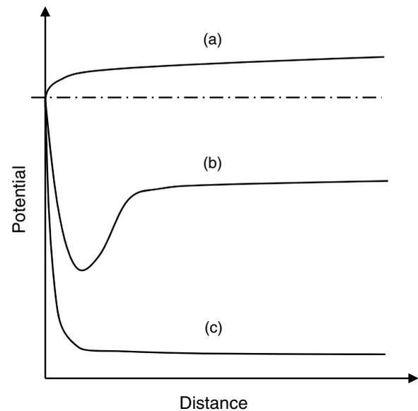
**Figure 2.** Sheath solutions for an electrode biased more positive than other plasma boundaries include (a) an ion sheath, (b) a double sheath and (c) an electron sheath.
