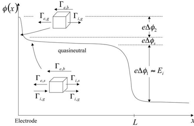
**Figure 9.** Schematic drawing showing the flux of ions and electrons entering and leaving Debye cubes in different regions of the anode spot.
