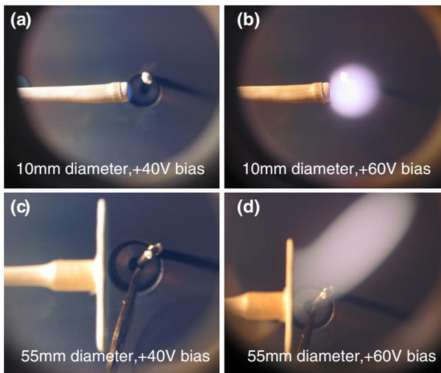
**Figure 1.** Photographs of equilibrium states of anodic double layers. Anode glows: (a) near a 1 cm diameter electrode and (c) near a 5.5 cm diameter electrode. Anode spots: (b) shows a fireball and (d) a firerod. The background shows an ion acoustic wave launcher and its holder that were not used in this experiment.
