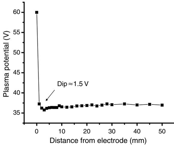
**Figure 10.** A double sheath potential profile (i.e. potential dip) measured with an emissive probe near an electrode biased at 60 V, which was supporting a firerod, but at a location away from the firerod.
