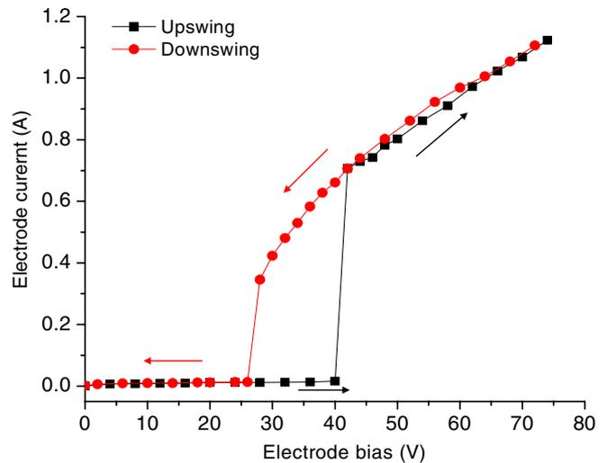
**Figure 6.**  $I$ – $V$  characteristic for a 1 cm diameter electrode taken increasing the electrode bias (squares) and subsequently decreasing it (circles). The data show hysteresis in the bias required for anode spot formation and disappearance.
