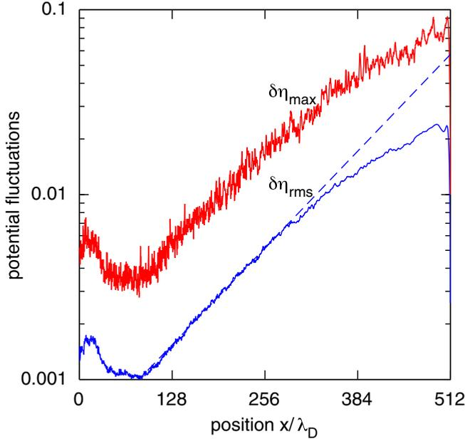
FIG. 6. Root-mean-squared (rms) (blue) and maximum (red) of potential fluctuations. The dashed line gives a linear spatial growth rate of  $0.0094/\lambda_D$ .
