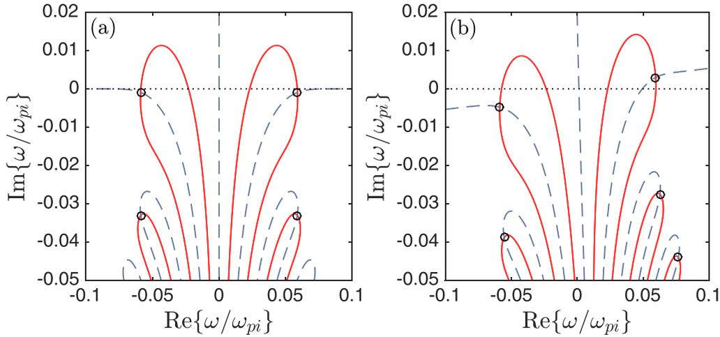
FIG. 9. Roots of the linear dielectric function from Eq. (20) with  $k\lambda_D = 0.05$ ,  $T_e/T_i = 10$ , and ion flow speed  $u_i = 0$ :  $\text{Re}\{\hat{\varepsilon}\} = 0$  (red solid lines) and  $\text{Im}\{\hat{\varepsilon}\} = 0$  (blue dashed lines). Circles are the crossing points, which represent the wave modes. (a) No electric field ( $E = 0$ ) and (b) with the electric field  $eE/(T_e/\lambda_D) = -0.001$ . The electric field leads to a growing mode.
