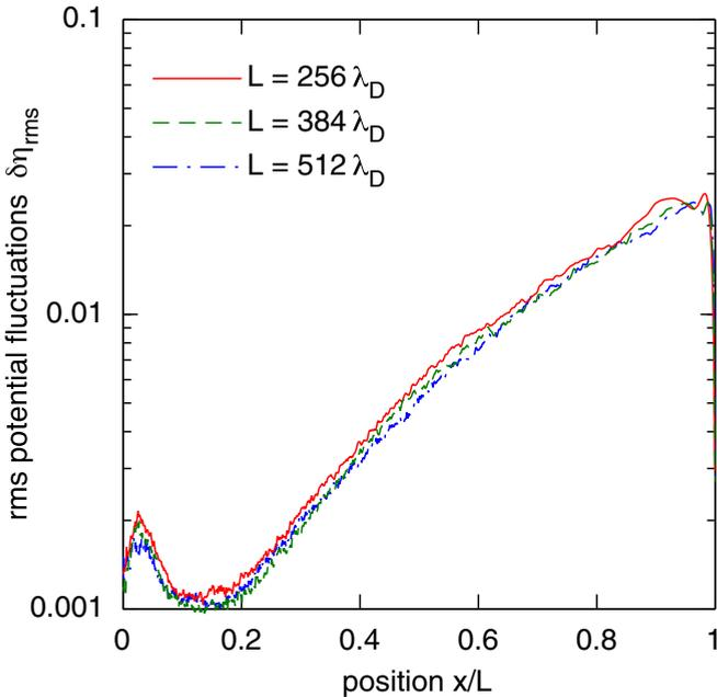
FIG. 7. Root-mean-squared (rms) potential fluctuations vs normalized position  $x/L$  for system lengths  $L = 256\lambda_D$ ,  $384\lambda_D$  and  $512\lambda_D$ . The spatial dependence of the fluctuations is effectively independent of  $L$ , indicating the fluctuations are a feature of the time-dependent TL model in the plasma approximation  $\lambda_D/L \ll 1$ .
