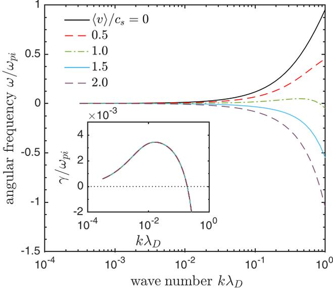
FIG. 11. Angular frequency and growth rate (inset) vs wave number for the linear dispersion relation computed from Eq. (20) with  $T_e/T_i = 10$  and  $eE/(T_e/\lambda_D) = -0.001$  at the five values of  $u_i/c_s$  indicated in the legend. All five curves are shown for the growth rate, but are indistinguishable, demonstrating that the growth rate is independent of the average ion velocity.
