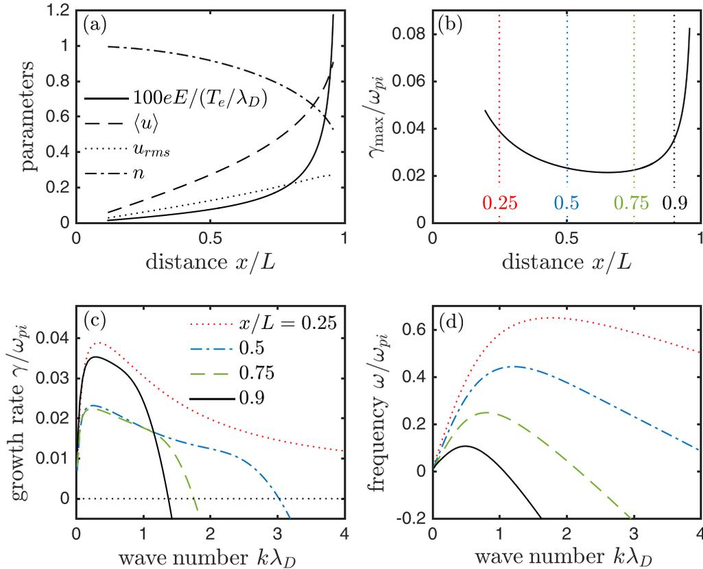
FIG. 13. (a) Profiles of electric field (solid line), ion flow speed (dashed line), rms ion speed (dotted line) and density (dash-dotted line) from the steady-state TL model (Ref. [15]). (b) The computed maximum linear growth rate computed from Eq. (20) using the parameters from panel (a). (c) Growth rate and (d) real frequency of the instability at the four spatial locations indicated in the legend.
