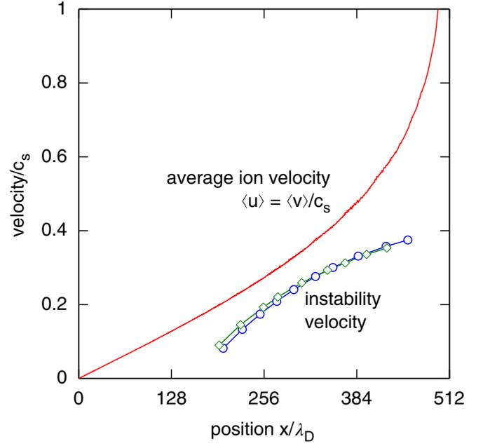
FIG. 5. The speed of unstable acoustic waves vs position  $x$ . The average ion velocity  $\langle v \rangle / c_s$  is shown for comparison. Speeds are normalized by the ion acoustic speed. The speed of the unstable waves is less than the average ion velocity, indicating that the unstable mode is propagating in the  $-x$  direction but is carried to the wall by the ion flow.
