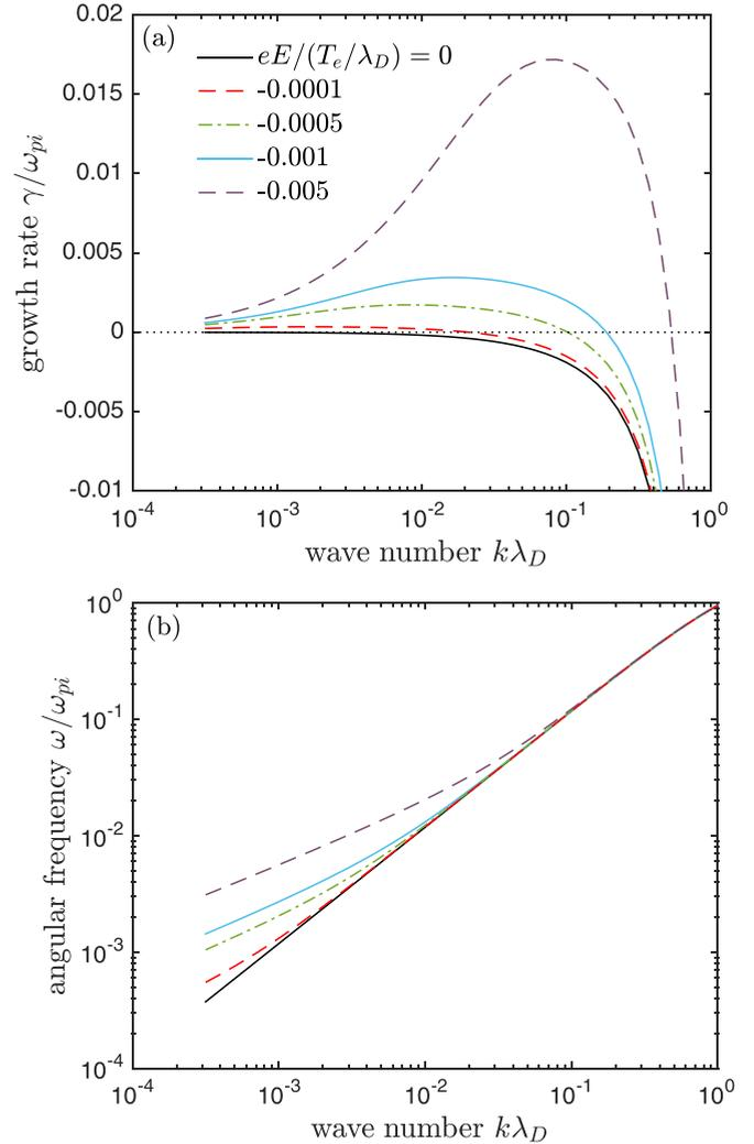
FIG. 10. (a) Growth rate and (b) real angular frequency of the linear dispersion relation computed from Eq. (20). The common data in each curve was  $T_e/T_i = 10$  and ion flow speed  $u_i = 0$ . The five chosen values of the electric field are indicated in the legend.
