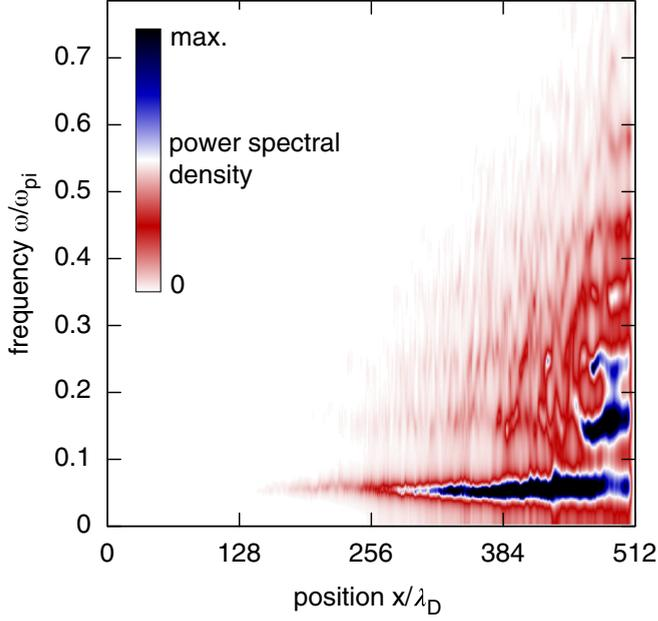
FIG. 3. Power spectral density (psd) vs distance from the center of the discharge and frequency normalized by the ion plasma frequency at the center of the discharge  $\omega_{pi}$ . A spectral peak with nearly constant frequency which grows with distance from the center of the discharge is found, indicating an unstable acoustic mode.
