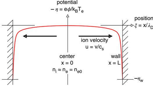
FIG. 1. Schematic of the Tonks-Langmuir discharge model. Cold ions are created and then accelerated to the walls by the self-consistent electric field.
